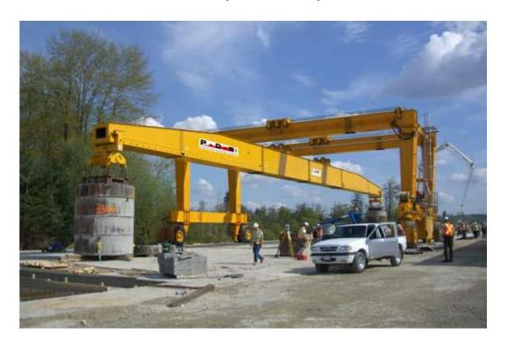
Client : GCJV Bilfinger & Berger Supplied equipment : Rubber tyred Straddle Carrier Capacity 300 t
